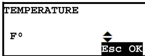
Select the mode by using the (▲)(▼) buttons and press START/OK (I) to confirm the setting. To cancel the operation press STOP/ESC (O).
