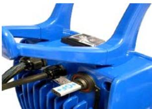
The USB type-A interface available on the rear of the machine is the main interface for communication purposes. Via USB, the user can download the protocols (fusion data) stored in the processor's memory as well as upload new software versions. The connector is protected against dust and water by a cap, which ensures an IP65 protection factor when properly screwed.
